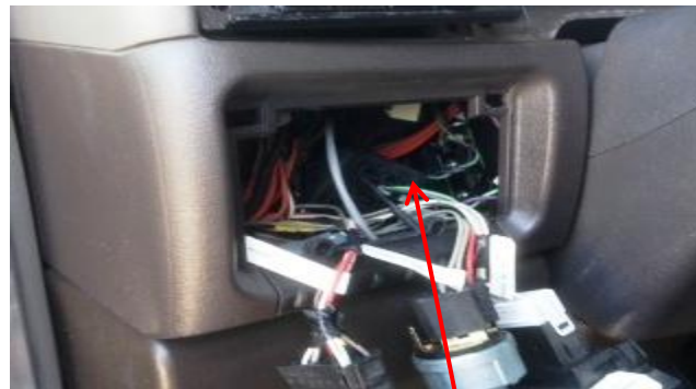
(Fig 3) Access to: J1587/J1708 Connector block
