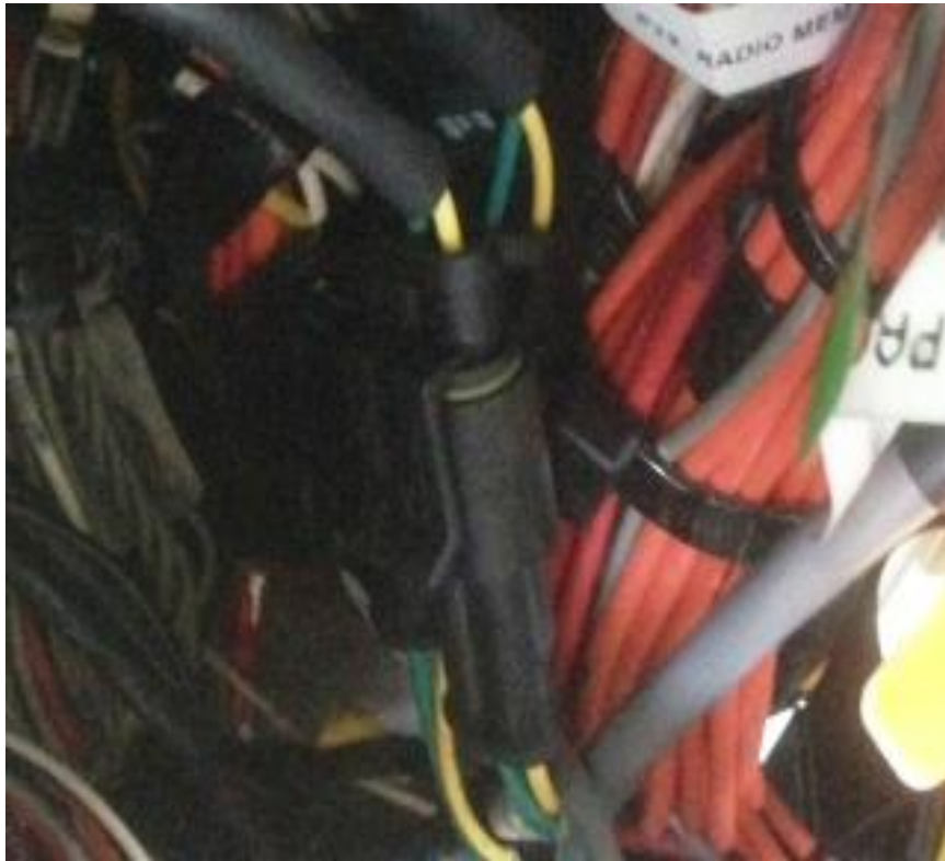
Fig (5) J1939 Super Seal connector Separate connector and join to DTY20687 Hydra cable mating connectors
