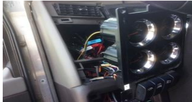
(Fig 2) Access to: pwr. gnd. ignition and J1939
